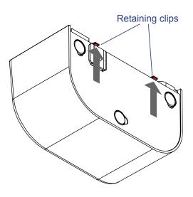
Simply push retaining clips towards fixed surface then slide PHASE off bracket
