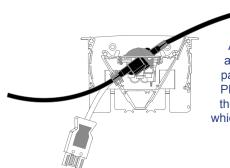
Angled data fascias allow data cabling to pass straight through PLATINUM, ensuring the integrity of cables which have a minimum bend radii (CAT5e, CAT6, etc)
